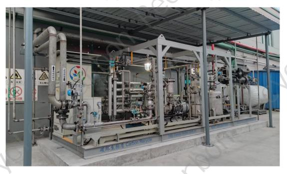
Fig. 8:Photo of 300Nm<sup>3</sup>/h methyl tert-butyl ether (MTBE) recovery equipment on site
