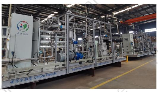
Fig. 11:Photo of 200Nm<sup>3</sup>/h N-hexane recovery equipment on site
