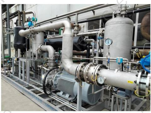
Fig. 1:Photo of 500Nm<sup>3</sup>/h Propanone waste gas recovery equipment on site
